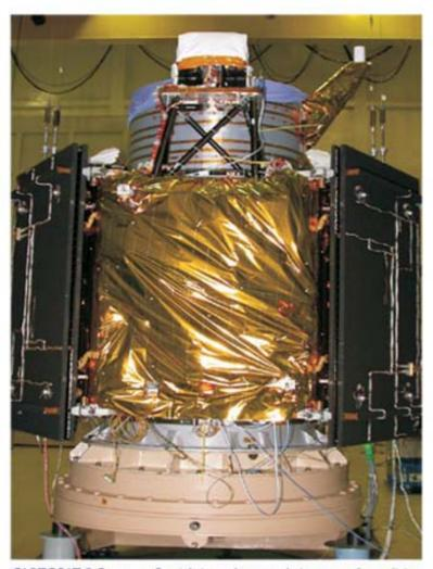
CARTOSAT-2 Spacecraft with its solar panels in stowed condition
